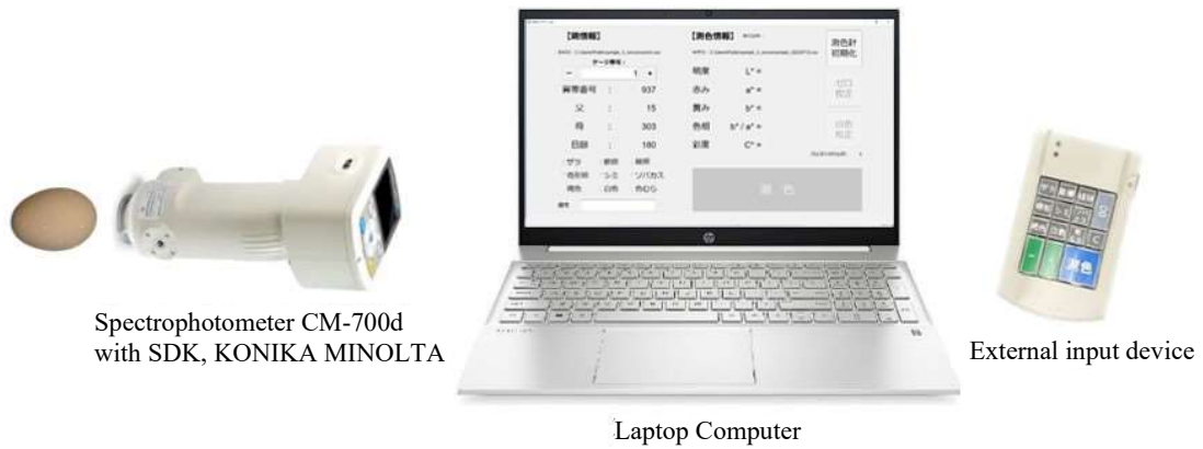
Figure 4: Prototype of the color visualization system for egg color
